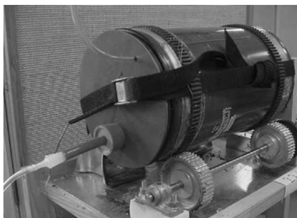
Figure 1. A composting reactor; a 3-l rotating Dewar vessel.
